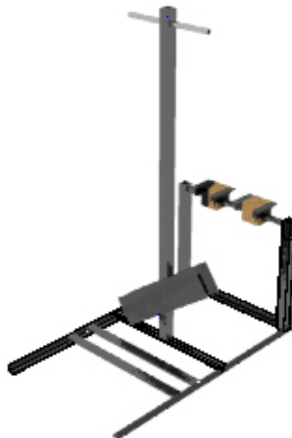
Figure 4.4: Frame with rocker arm and treadle pivot system
