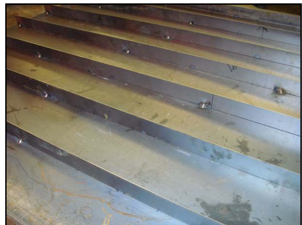
Figure 27. Top of solar collector with fins
