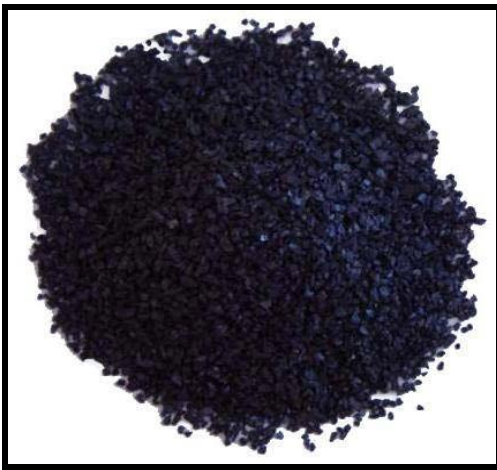
Figure 15. Granular activated carbon
