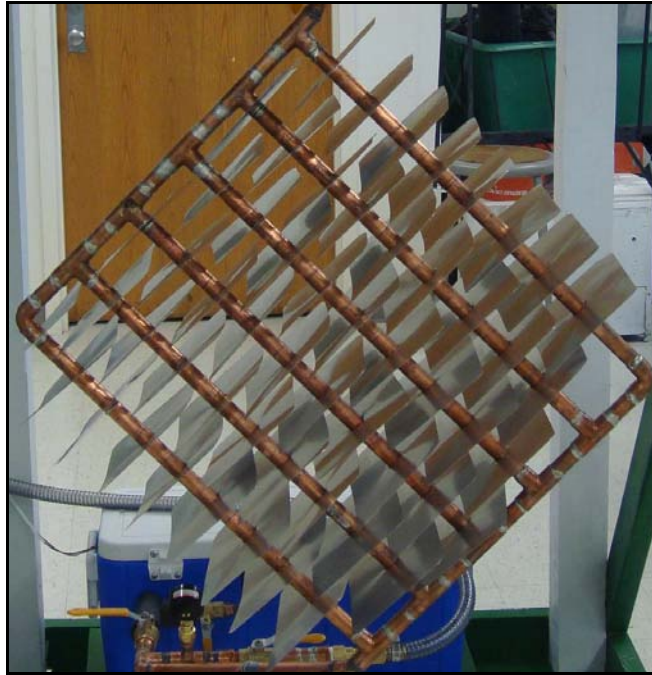
Figure 25. Completed condenser with fins attached.
