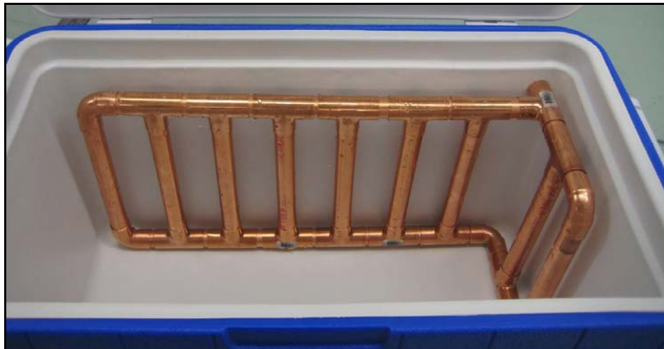
Figure 24. Completed evaporator in cold space to locate hole.
