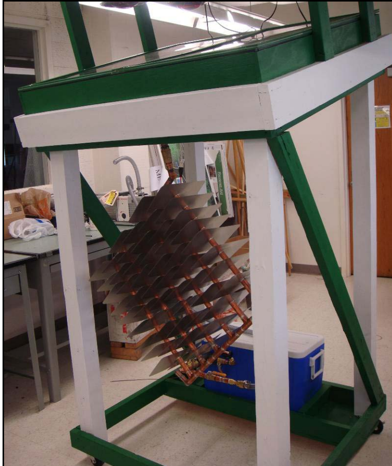
Figure 28. Completed assembly of adsorption refrigerator.
