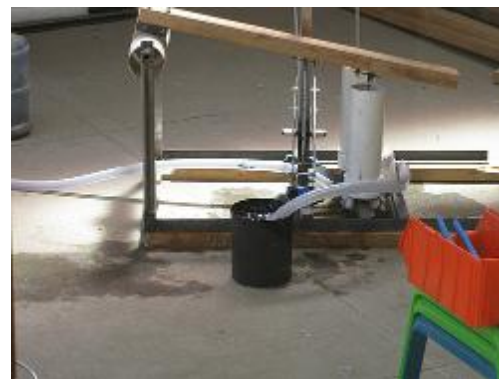
A treadle pump designed for rural people in Tanzania. (John Barrie)
